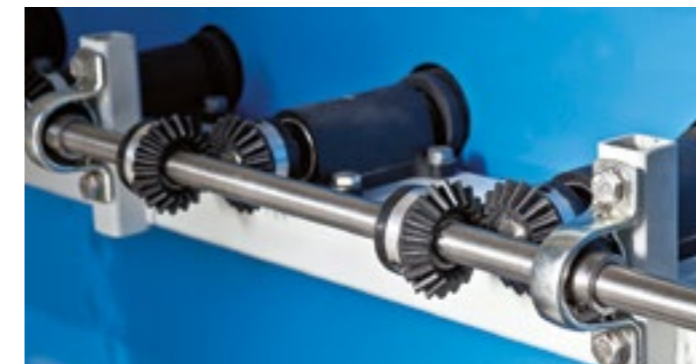
Glass conveying system with rubber scratchproof rollers, driven by maintenance free conical gears. Mechanical transmission in stainless steel. Axes of the conveying rollers and of the brushes made in stainless steel.
