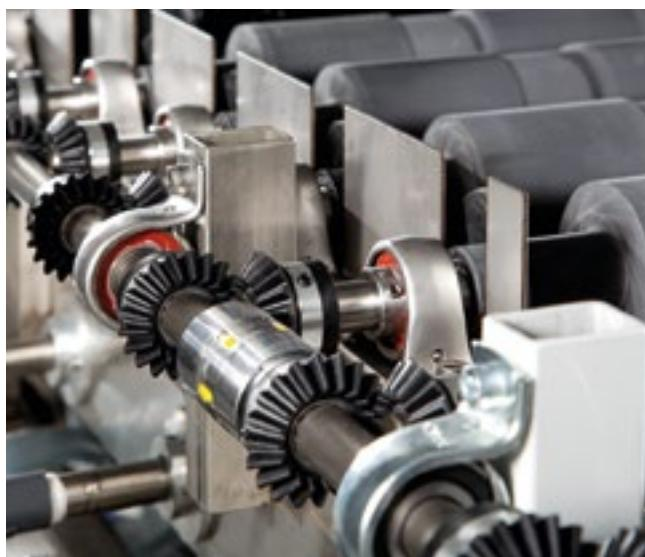
Transmission with conical gears in reinforced PA6, driven by a shaft in stainless steel, maintenance free. Shaft covered up to the hub.
