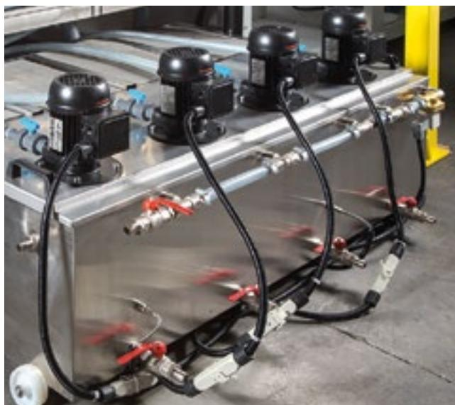
Possibility to heat the water and maintain the temperature up to 60 ° C with resistances, thermostats and resistance protection sensors. Removable and compact tank in stainless steel for minimal encumbrance and easy maintenance.
