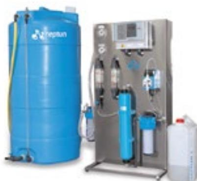
**DEMI** series Demineralization units. Demineralization unit, with reverse osmosis, up to three stages, for the production of demineralized water. Available with different production capacity: from 30 l/hr to 190 l hr.
