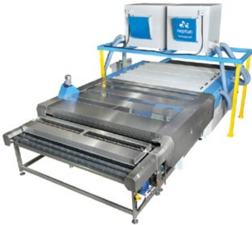
**Tornado HP** is equipped with a powerful PLC with touch screen allowing the management of numerous advanced functions, for glass sheets with thickness up to 38mm. Thanks to the high level of automation and flexibility, there are no limits for integration into all existing production lines.
