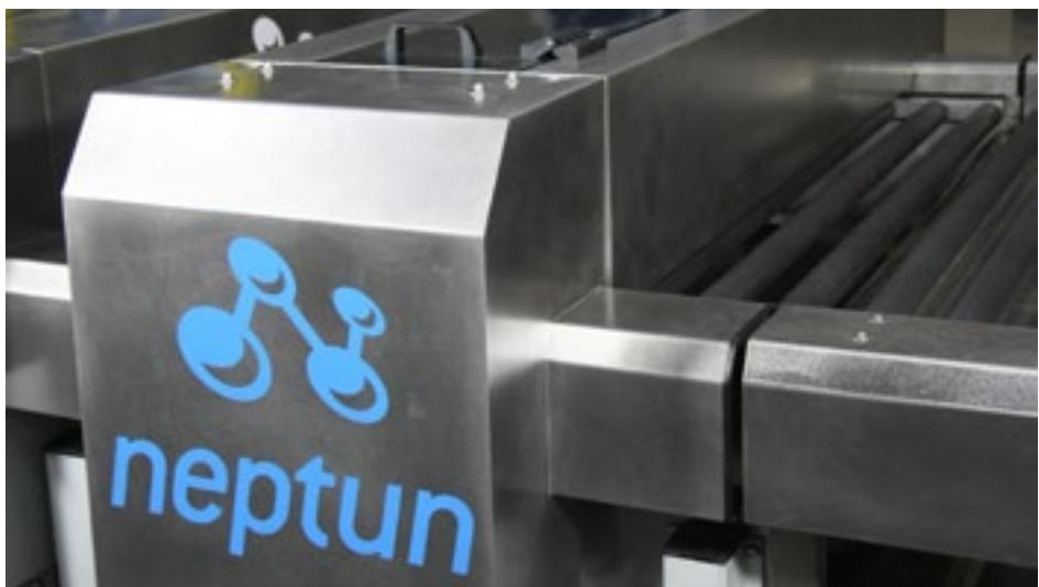
The additional prewashing module with brushes is complete with top and bottom brush, tank and pump, fan and upper air knife. Particularly suitable for very dirty glasses that require an aggressive pre-wash.
