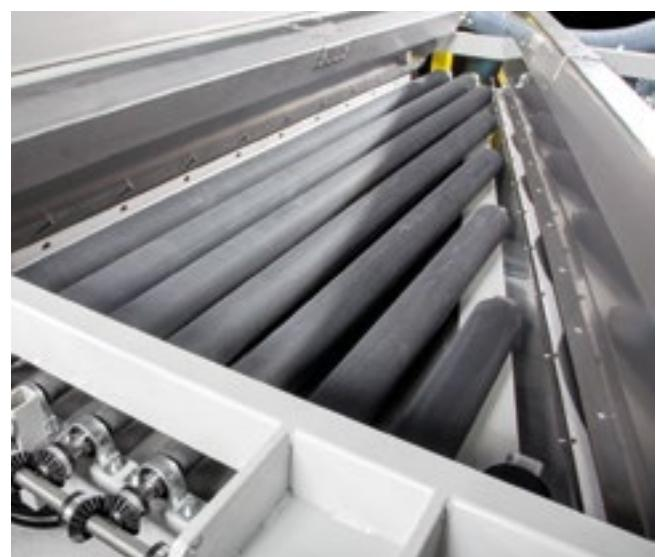
Washing area and drying blades in stainless steel. Air knives and water collecting slide in stainless steel.
